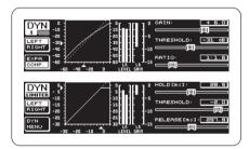
Everything you'd find on a dedicated compressor/expander is here including variable rations from 1:1.1 to 1:100, ATTACK times from 0 to 200ms, 0-3dB variable knee and 20 to 4000ms RELEASE, all adjustable from a coarse/fine adjustment scale. The built-in separate LIMITER has Threshold, Hold and Release functions.
